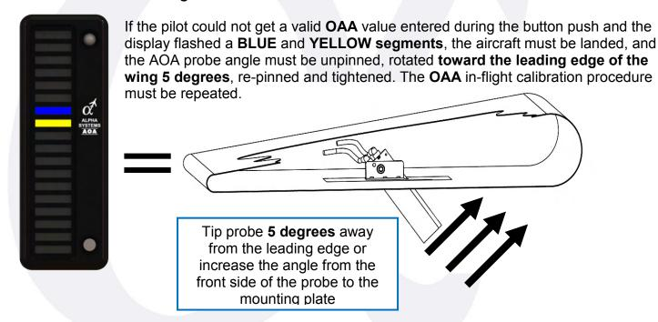
Note: The CAL Button can be pushed as many times as desired to continuously attempt a new Optimum Alpha Angle (OAA) set-point. If the set-point is valid the display will be functional using the new OAA value. If the set-point is invalid, the display will no longer be operational and continue to flash the error colored backgrounds. As long as the unit is in the OAA CAL routine, it will flash the blue segment twice, every five to six seconds until you enter Cruise Calibration.
