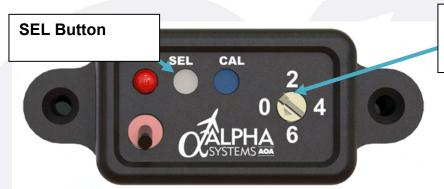
Rotary Switch in Setting Number 1 for Zero Offset Calibration
